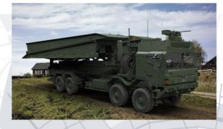
Furthermore, the COBRA, a modular armored front launched bridge system can be mounted either permanently or temporarily and launched and retrieved in under 4 minutes. The medium-weight wheeled or tracked carrier vehicles maintain their primary functions, while offering multi-functional bridge capabilities whenever needed, thus ensuring highest operational flexibility at all times.
