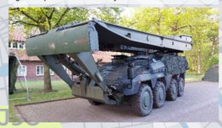
In the field of special bridges, GDELS-Bridge Systems developed the VIPER, an MLC40 Modular Trackway Bridge for gap crossing up to 5, 7 or 9 meters.
