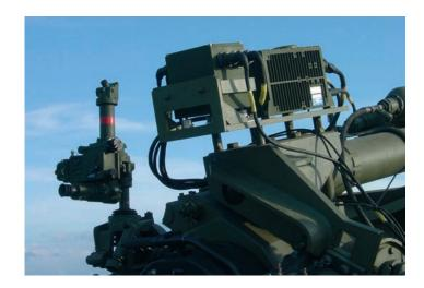
DINAPS is a modular and customizable system, combining a hybrid (Inertial+GPS) Navigation System, a Muzzle Velocity Radar (MVR) and powerful Software solving in real time the ballistics for static or moving targets and for any combination of projectile-charge available.
