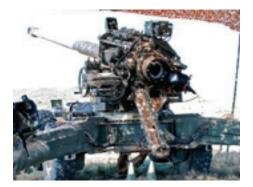
The SIAC is a state-of-the-art 155/52 caliber towed howitzer with selfpropelled capabilities due to its integrated auxiliary power unit.
